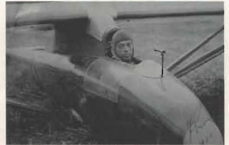
Fig 10. Robert Kronfeld in his Wien. The double curvatures of the cockpit were made by skinning with small pieces of plywood.
