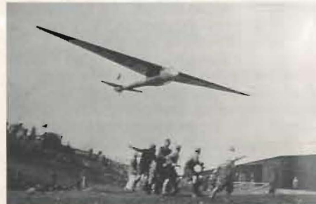
Fig 18. The Rhönadler being bungy launched. It was one of four gliders to fly the first 500km on July 19, 1932.
