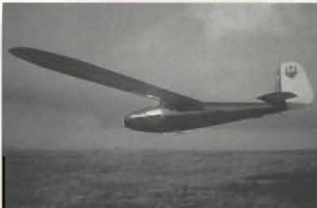
Fig 7. The Darmstadt Akaflieg D-15 "Westpreussen" of 1926 developed the classic configuration of the high performance glider.
